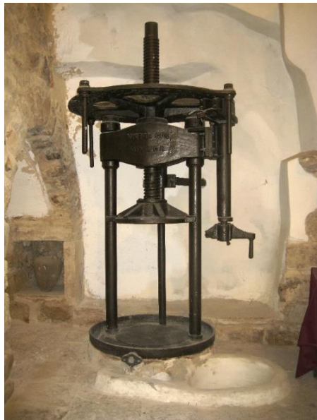
Figure (14): Victor Coq manual iron-screw press at an-Natsha, family ma'sara. Photo
