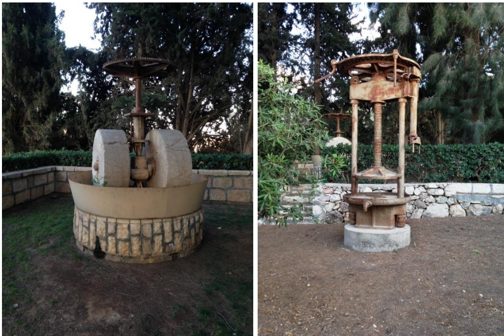
Figure (35): crushing installation (left). Figure (36): Victor Coq’s French-made manual iron screw press (right). Photo © Maissoun
